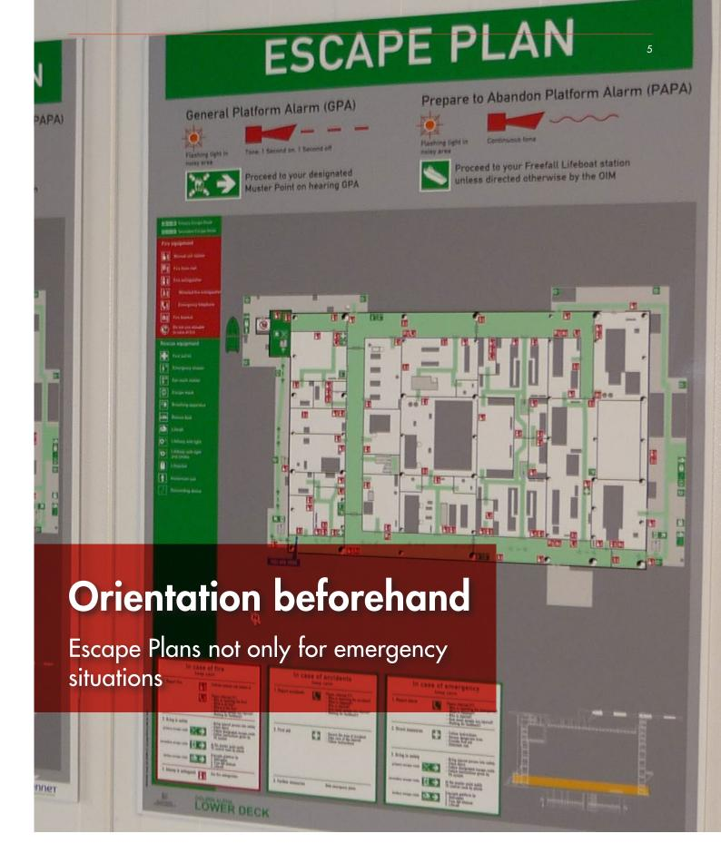
Regardless of a person's location on a ship or offshore installation, rapid evacuation must always be possible. Unambiguous communication in the escape route marking under every circumstance is extremely important. It must always be possible to find and recognize the various applicable escape routes at a glance. In addition to an escape route marking system, comprehensive escape plan signboards help to orientate in controlled and uncontrolled situations.
